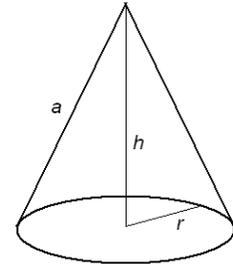
Solution: There is a right triangle formed by  $a$ ,  $h$ , and  $r$  as the picture shows. We state the Pythagorean theorem for this triangle and solve for  $h$ .
