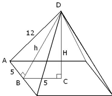
$$\begin{aligned} (5 \text{ m})^2 + h^2 &= (12 \text{ m})^2 \\ 25 \text{ m}^2 + h^2 &= 144 \text{ m}^2 \\ h^2 &= 119 \text{ m}^2 \\ h &= \pm\sqrt{119 \text{ m}^2} \implies h = \sqrt{119} \text{ m} \end{aligned}$$
