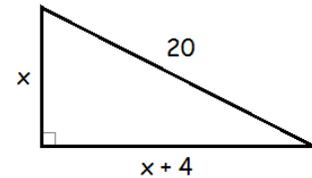
$$\begin{aligned} x^2 + (x + 4)^2 &= 20^2 && \text{expand } (x + 4)^2 \\ x^2 + x^2 + 8x + 16 &= 400 && \text{combine like terms} \\ 2x^2 + 8x + 16 &= 400 && \text{subtract 400} \\ 2x^2 + 8x - 384 &= 0 && \text{factor out 2} \\ 2(x^2 + 4x - 192) &= 0 && (x + 2)^2 = x^2 + 4x + 4 \\ 2(\underbrace{x^2 + 4x + 4}_{(x+2)^2} - 4 - 192) &= 0 && \\ 2((x + 2)^2 - 196) &= 0 && \\ 2((x + 2)^2 - 14^2) &= 0 && \\ 2(x + 2 + 14)(x + 2 - 14) &= 0 && \\ 2(x + 16)(x - 12) &= 0 && \end{aligned}$$
