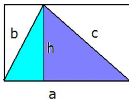
Our triangle makes up for half of a rectangle, with sides  $a$  and  $h$ . Thus  $A = \frac{ah}{2}$  ■
