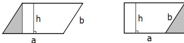
Thus the area of the parallelogram equals to the area of a rectangle with sides  $a$  and  $h$ . ■
